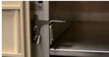
Easy release handle to open master gate
